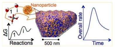
Schematic of the new Kinetic Monte Carlo algorithm and resulting rate curve
